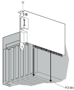
Figure 2-2. Installing the adapter in a server
